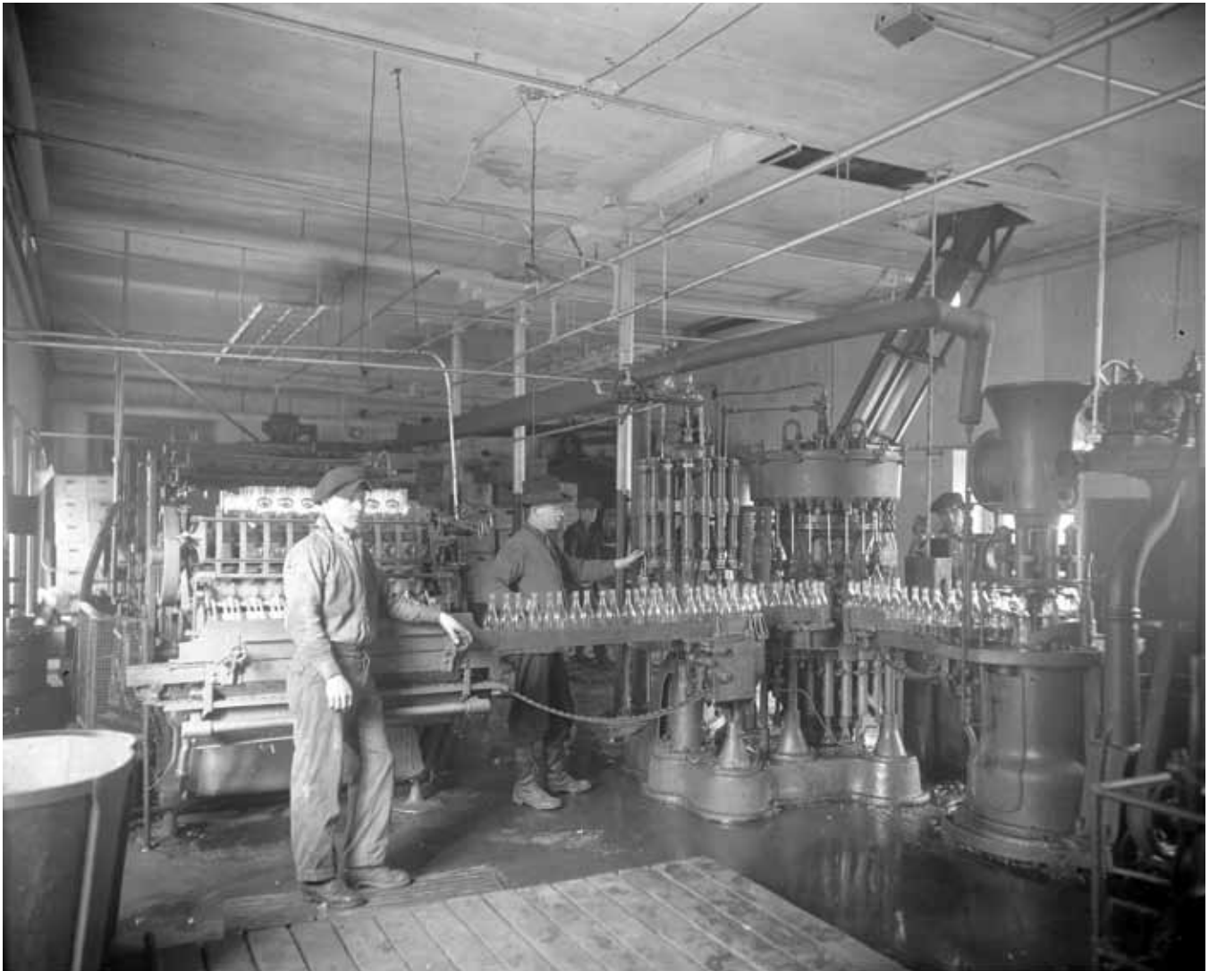
Fig. 23. Workmen washing, filling and crowning mineral water bottles in November 1918 in a plant run by the New York State Conservation Commission in the New York State Reservation, now Saratoga Spa State Park, near Saratoga Springs. Photo: New York State Archives, 14297-87, SARA No.375.
