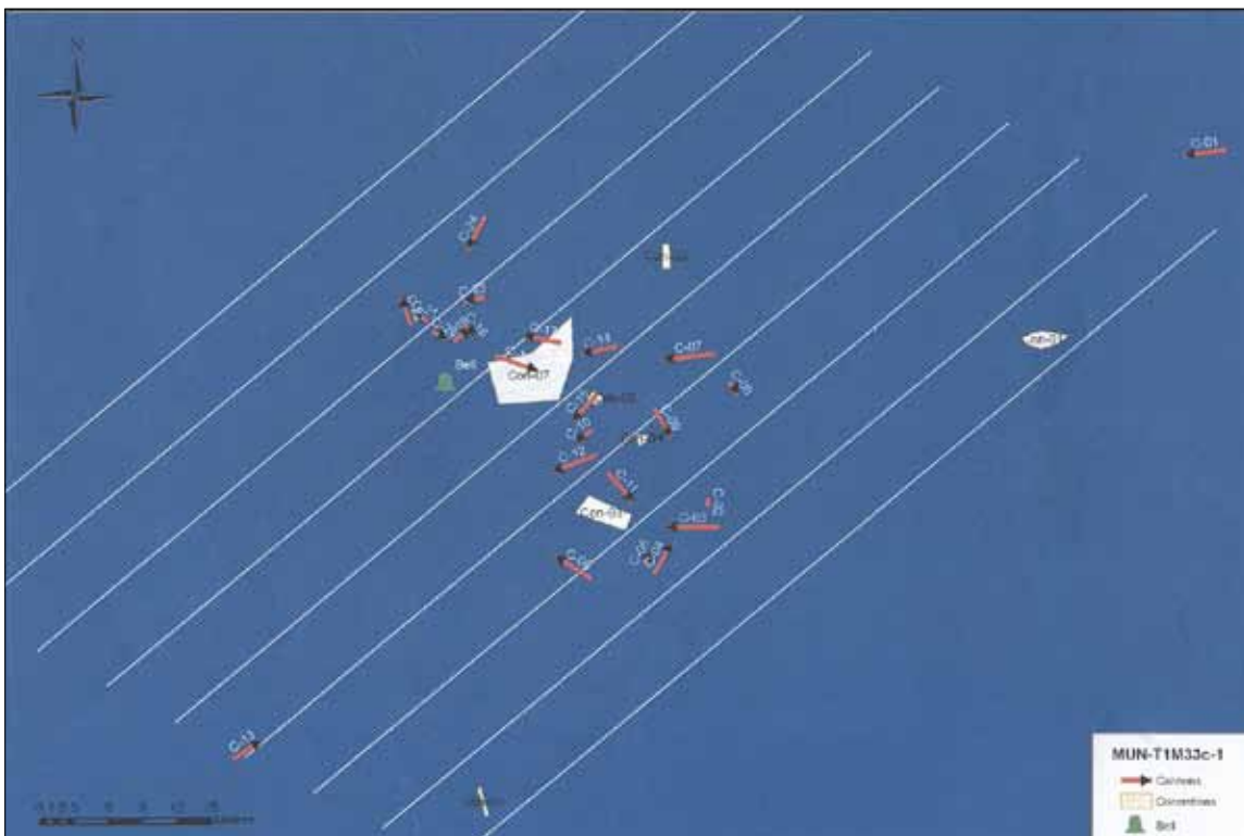
Fig. 4. An electronic grid with 5m spacing intervals, running northeast to southwest, was established for the ROV Zeus to survey Site 33c systematically.
