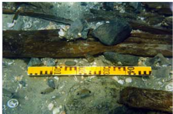
Fig. 4. Tenons on the hull of the late 6th century Dor D shipwreck were left loose in mortises and were unpegged. The same harbor has yielded 6th-century wrecks that are of entirely frame-first construction. The commercialization of the Holy Land wine trade was a major stimulus behind the shift away from shell-first shipbuilding. Photo: Sean Kingsley.
