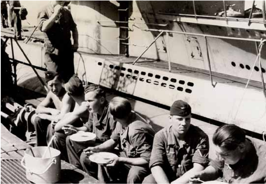
Fig. 20. Crew members taking a meal on the deck of U 1021 (front) alongside a sister boat from the same building yard in harbour while working up in the Baltic Sea, presumably at Pillau during autumn 1944. The crew members are sitting on top of the schnorkel tube laid down on deck. The cooking pot forward left is standing on the cover grating shown in Fig. 18.
