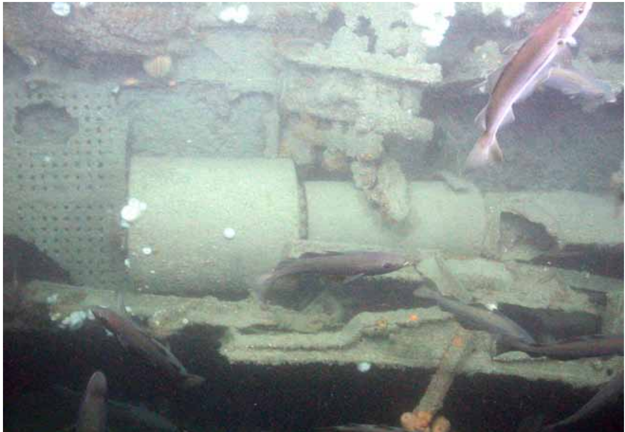
Fig. 4. Schnorkel head lying on the deck of wreck of U 325, with the cylindrical part covered with Jaumann-type anti-radar camouflage.
