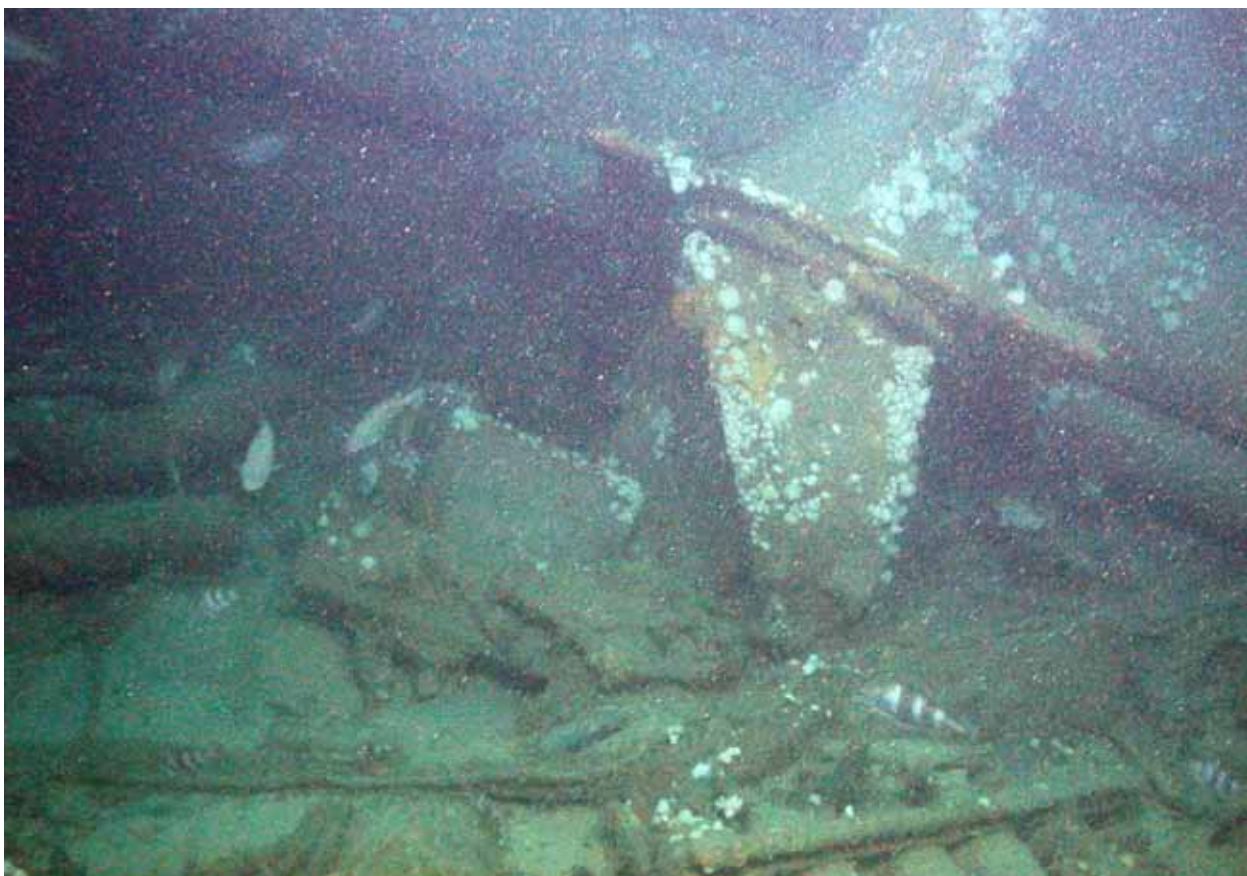
Fig. 15. A late-war Type LM43U gun mount, complete with a 3.7cm M42U AA-gun lying on the seabed beside the wreck of U 1021 (site D). The gun mount is inverted with the gun breech present just above the sandy sea bottom. The crew protection shield has already fallen off.
