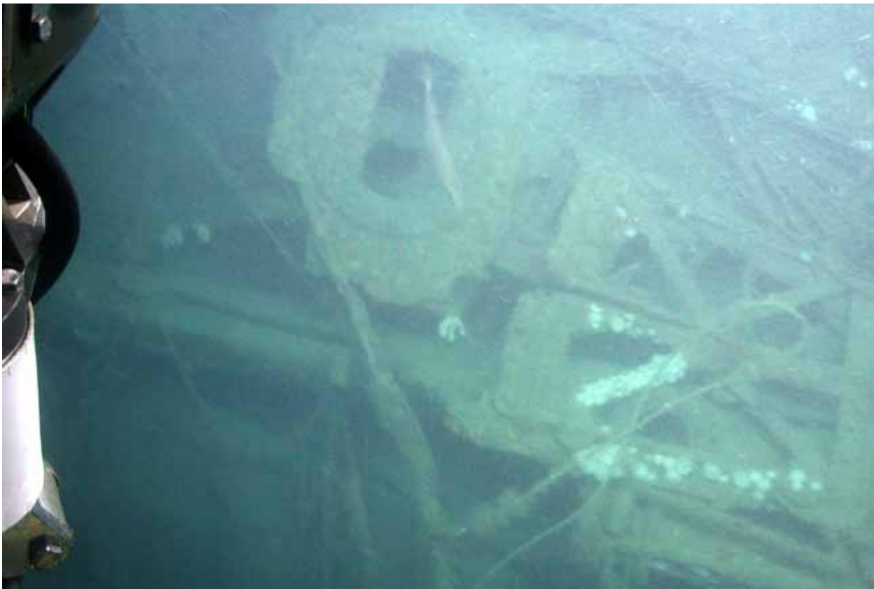
Fig. 7. The massive gun mount for the 8.8cm deck gun features prominently on the wreck of U 650. Beneath is the lower part of the schnorkel mast lying on the deck. The circular opening of the pressure flange connecting to the fresh air intake tube, characteristic of the older Type 1 schnorkel installation, is partly obscured by the rectangular wooden deck cover of the former 8.8cm ready ammunition store located just behind the gun mount.
