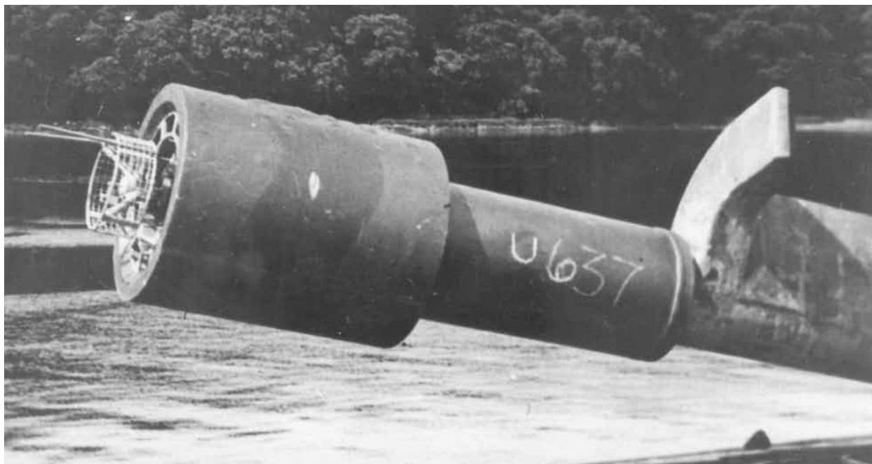
Fig. 5. View of the ring-float schnorkel head installed on U 637 taken post-war at Lisahally, Northern Ireland, displaying a Jaumann anti-radar absorber used to camouflage the schnorkel head against radar detection, comparable to that installed on U 325. The layered absorber measured about 7cm in thickness. On top of the schnorkel head the 'Bali I' -detector antenna, used against metric radar sets, can be seen, which, however, were hardly in use any more in 1945.
